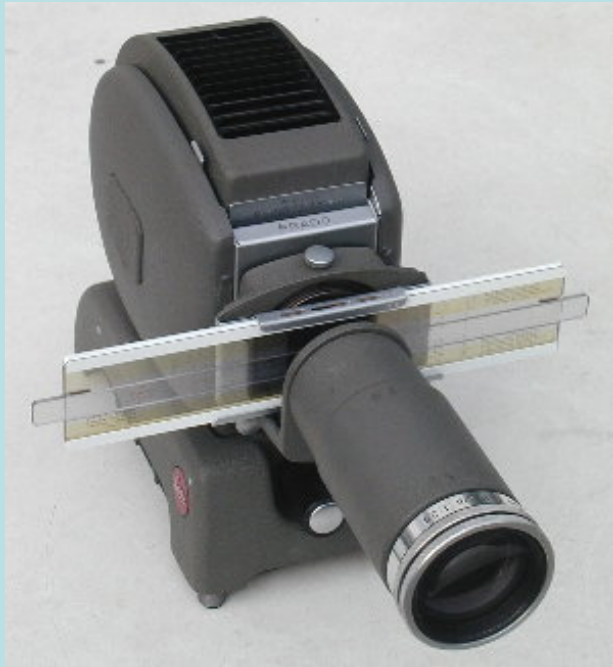
Aristo 203 Scholar projection slide rule for the classroom mounted on Leitz Prado slide projector
